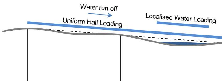
Figure 7: Accumulated Hail and Water Loading on Roof
