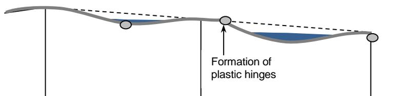
Figure 8 – Formation of plastic hinges leading to collapse
