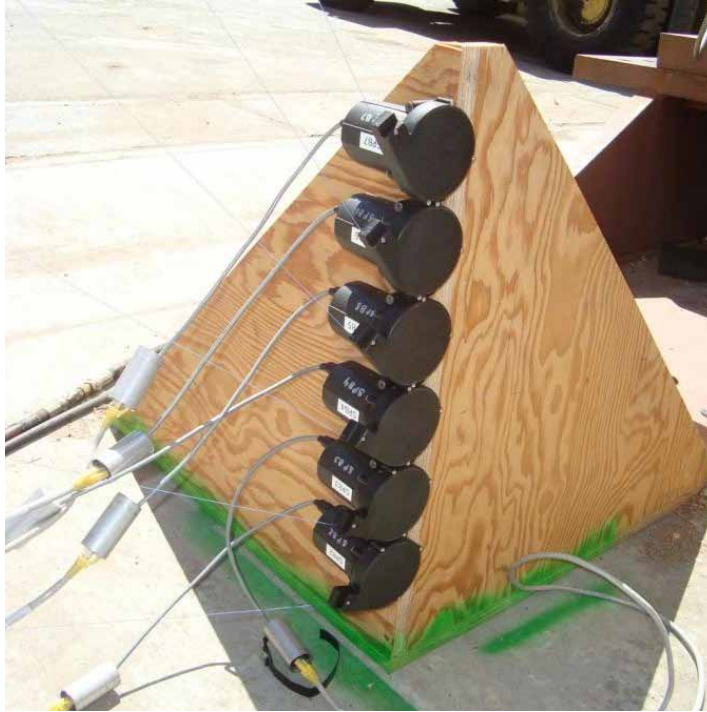
Figure 3.65: South fixed point of the string pots
