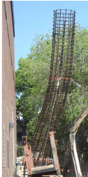
Figure 3.70: Specimen I deformed shape, view from South
