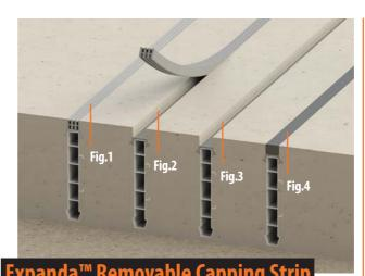
PaveX™ Expanda™ profile is supplied pre-fitted with a durable, stay-in-place capping (Fig. 1).
